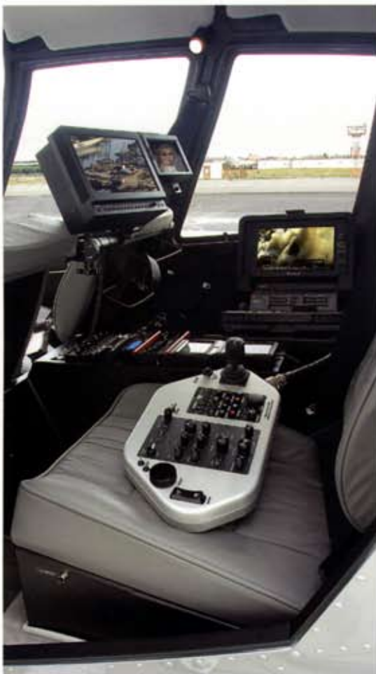
TOP The digital age has allowed all the ALE gear you could want to fit nicely in the cockpit of the R44.
